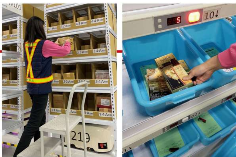
(左) 倉儲人員將貨品上架至無人搬運車 (AGV) 貨架。 Warehouse staff using an AGV. (右) 倉儲人員於 CAPS 理貨站透過電子標籤揀貨、分貨。 Warehousing personnel handling goods using electronic tags at a computer-aided planning and scheduling (CAPS) tally statio.
